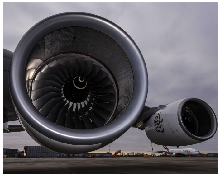
Figure 17: Novel nacelle acoustic technologies – industry-first acoustically spliceless acoustic inlet on A380 / Trent 900.
