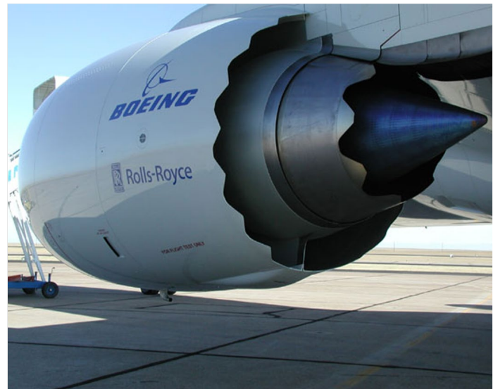
Figure 15: Quiet Technology Demonstrator Engine, showing Nozzle Treatment options on a 777-200ER with Rolls Royce Trent 800 Engines.
