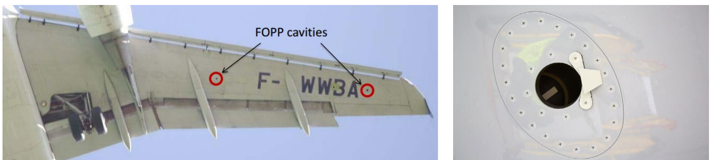
Figure 19: Left: Red circles indicate Fuel Over Pressure Protector (FOPP)cavities locations. Right: Air flow Deflector installed next to a FOPP cavity, eliminating generation of tonal noise during flight.
